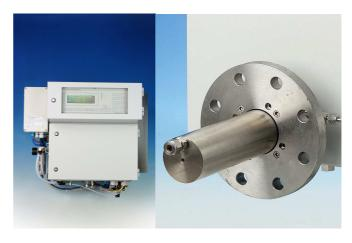
Der Thermo FID-MK II 2/3G Ex pz II Zone 2 following ATEX 94/9/EG is an accredited Zone 2 application. With a measuring head attached directly without any filter or sample gas conditioning to a DIN gauge connection. Over a status signal or by the remote control function it is possible to control and see the analyser function in real-time. The housing is in protection class IP65. (Exhaust Emission control; Plant monitoring)
